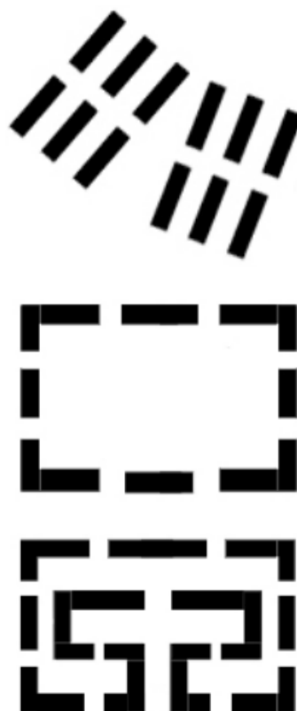
[Fig. 9] Residential block shapes (drawn by the author according to an actual survey : row block [left], perimeter block [center], double-perimeter block [right]).
