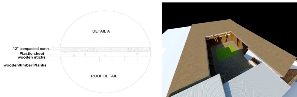
Figure 19. Roof top and Typical Section of a roof and highlighting the details in slab
